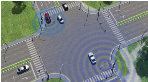
The system allows cars to talk wirelessly with one another using DSRC on a secure FCC-approved channel
