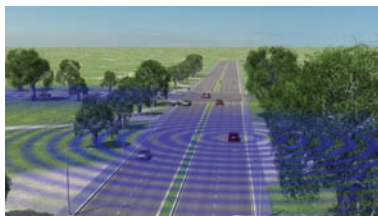
The system allows cars to talk wirelessly with one another using DSRC on a secure FCC-approved channel
